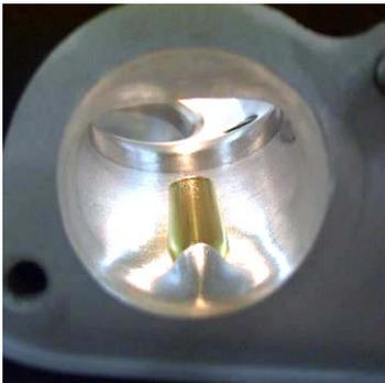
Though a reasonably priced package the XB SS1.0 gets the full treatment, at left is the finished intake port with optional manganese bronze valve guides installed. At right is the Serdi applied 5 angle/radius seat cuts after complete port work but before the final chamber and port blending.
