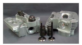
The E80SS1.1 package is performed to customer supplied stock castings and includes EV8 stainless steel valves, heat treated cast iron or bronze manganese guides and hi-lift valve springs. The ports are thoroughly contoured and proprietary multi-angle valve seat geometry is applied. The finished product is a completely blue-printed assembly. Manifold matching and decking are optional.
